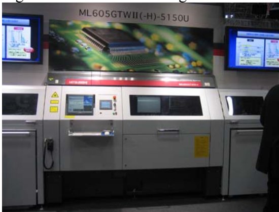
Figure 17. Mitsubishi Electric 4-Beam CO 2 laser.
