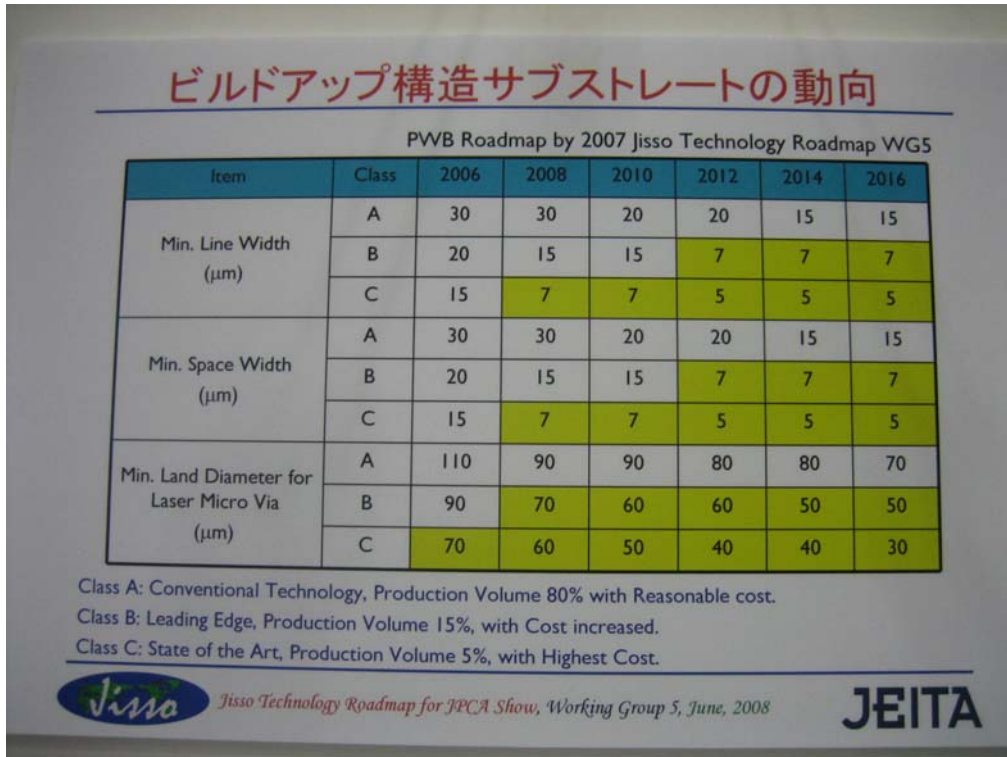
Figure 29. Technology Trend of Build-Up IC Substrate.
