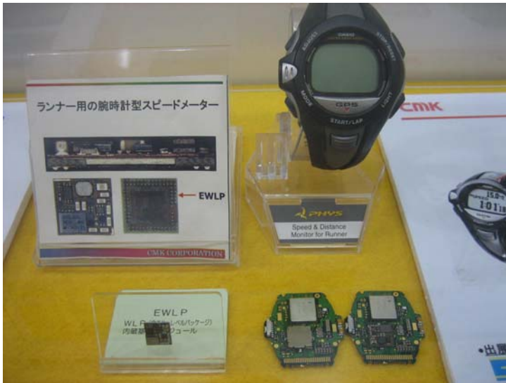
Figure 7. CMK showed an example of wafer level package integration for watch module.
