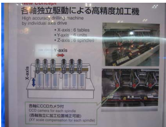
Figure 20. Six-spindle HVM version of the independent axis drive machine.
