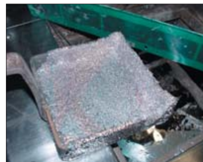
FIGURE 5. Tin-copper needles being removed from solder by a skimming tool.
